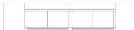
Tray Layout in Standalone Ice Cream or Pastry Area tray: 1060 x 400 mm
